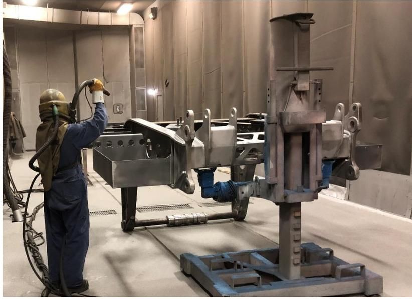
A large electrical and air source atomizes the aluminum and zinc metal into a spray. This spray travels to the metal surface where it instantaneously solidifies when it contacts the cool metal. The two metals are now mechanically bonded together.
